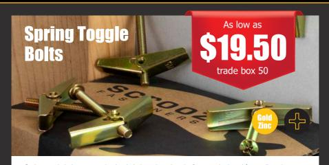
Spring toggle bolts are a spring loaded plasterboard cavity fastener designed for medium duty applications into hollow walls or hollow wall sections. They work by way of expansion, the spring loaded wing portion of the anchor is folded and inserted into the plasterboard wall or cavity, on tightening the cavity the wings expand against the inside of the cavity wall. Phillips No 2 drive.
