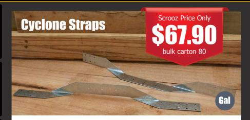
Cyclone straps are used to secure rafters and trusses to top plates, purlins and beams as a general fixing or in areas with cyclonic, or high wind conditions to help prevent lift. They are flexible high strength timber tie down connectors, easy to bend around rafters and beams. Made from 1mm galvanised steel with 3.4mm pre-punch holes for quick and simple installation.
