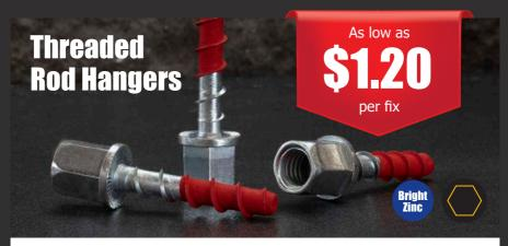
Self tapping rapid fix screw in masonry anchor with an M10 internal thread that allows 10mm rod or bolts to be hung from ceilings to hang ductwork, cable tray and services from concrete ceilings. Quick and easy to install and fully removable, tapered end for easy insertion into predrilled hole. Optimised thread pitch for increased installation speed and serrated flange head for improved grip. Bright zinc plated for corrosion protection, drive socket also available.
