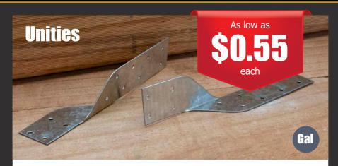
Unitie connectors are strong and economical brackets used for joining timber crossing at right angles. They can be used anywhere a timber connection is required and are a simple, fast solution for purlin anchors and truss or rafter tie-downs. Made from 1mm galvanised steel in left and right-hand versions with 3.4mm pre-punch nail holes, 170mm long.
