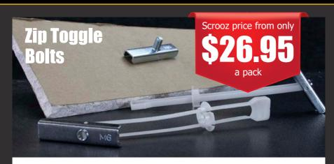
Rapid Fix Zip toggle bolts cavity wall anchors are a fast and strong solution for medium to heavy duty general purpose fastening of fixtures to plasterboard cavity walls, ceilings and general hollow structures and components. Requires a minimum cavity of 50mm. The nylon arms are for installation purposes only and snap cleanly off once the zip toggle bolt fastener is in place. Uses a 6mm threaded bolt or screw (not supplied).
