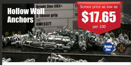
Hollow Wall Anchors are expansion cavity fixings used to fasten fixtures to plasterboard walls and other board materials where a cavity is present. The clamping action provides a very strong anchor point spreading the fixture load by deforming to an umbrella shape behind the board and preventing pull-through when tightened, includes captive phillips drive low profile zinc plated roundhead screw.
